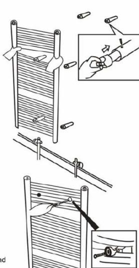
7 Offer the ladder rail A up to the fixing brackets and place bolt J through the bracket bush K.
