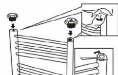
3 Thread the tails from the valves (not supplied) into the bottom two threads. Apply PTFE tape.
