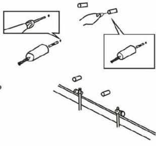
6 Place the spacer H inside the wall support and insert the small screw G into the hole in the wall support. Don't over-tighten to allow for adjustment later.
