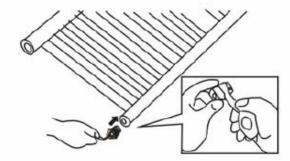
4 The wall supports should be fitted at approximately 10cms from the inside edge of the ladder rail - 2 near the top of the ladder rail and 2 near the bottom. The mounting height can be varied between any of the ladder rail bars to allow for finding the best fixing point on the wall. Mark the fixing points with a pencil.
