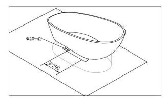
2.Install the drain and plumbing pipe and fixing of pop-up part
