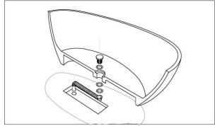
3. Align the drain to the expansion joint, apply sillcone to between of them.
