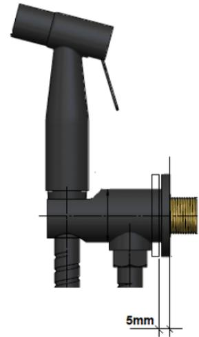
Wall plate tolerance of 5mm
