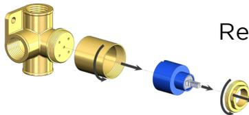
Remove MW13-BDY components
