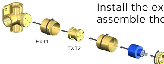
Install the extension sets and re-assemble the MW13BDY components
